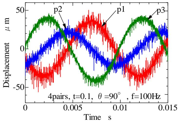
Figure 5. Behavior of vibration plate ( $f=100\text{Hz}$ ,  $\theta=90^\circ$ )
