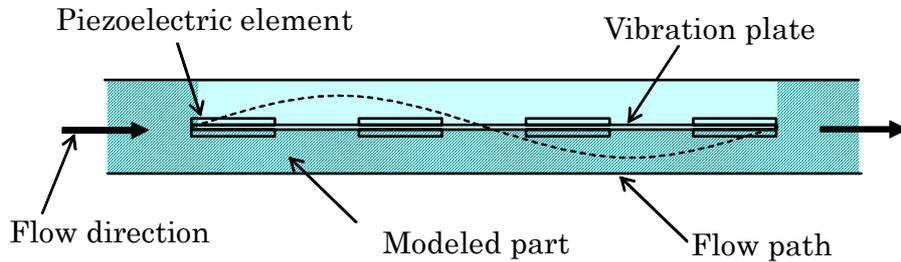
Figure 9. Schematic view of flow path cross section
