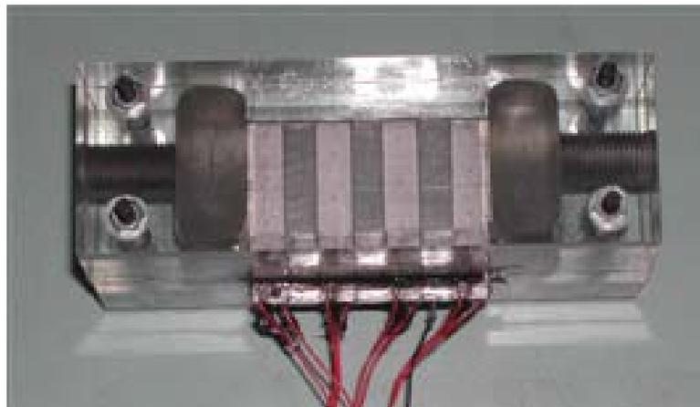
Figure 4. Schematic view of the experimental pump assembly
